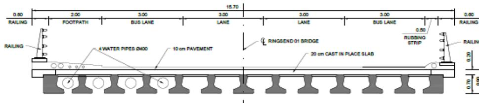
**Figure 8-3: Deck Section Ringsend 01**
