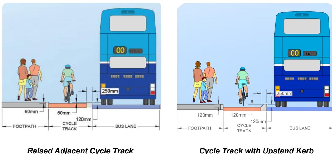
**Figure 4-5: Fully Segregated Cycle Track**
