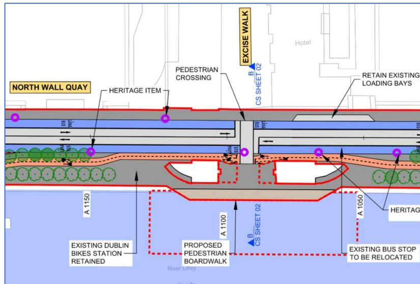
**Figure 3-9: Proposed Layout on North Wall Quay with Proposed Boardwalk on the River Side**
