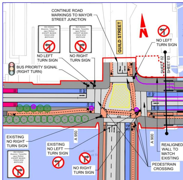
**Figure 3-10b: Proposed Traffic Turn Restrictions at Guild Street Junction**
