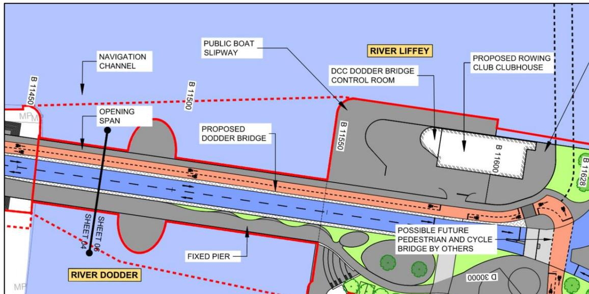
**Figure 3-18: Plan of the proposed River Dodder Public Transport Opening Bridge**
