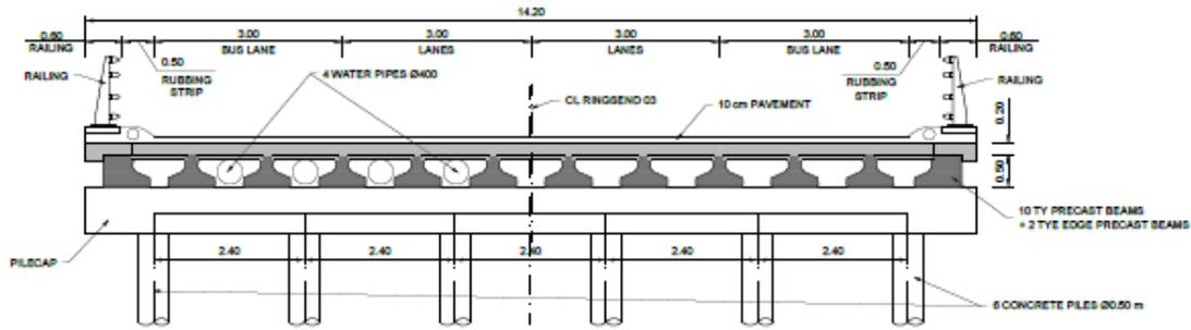
**Figure 8-12: Abutment Section Ringsend 03**
