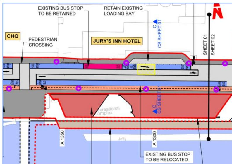
**Figure 3-6a: Proposed Road Layout at Custom House Quay West**
