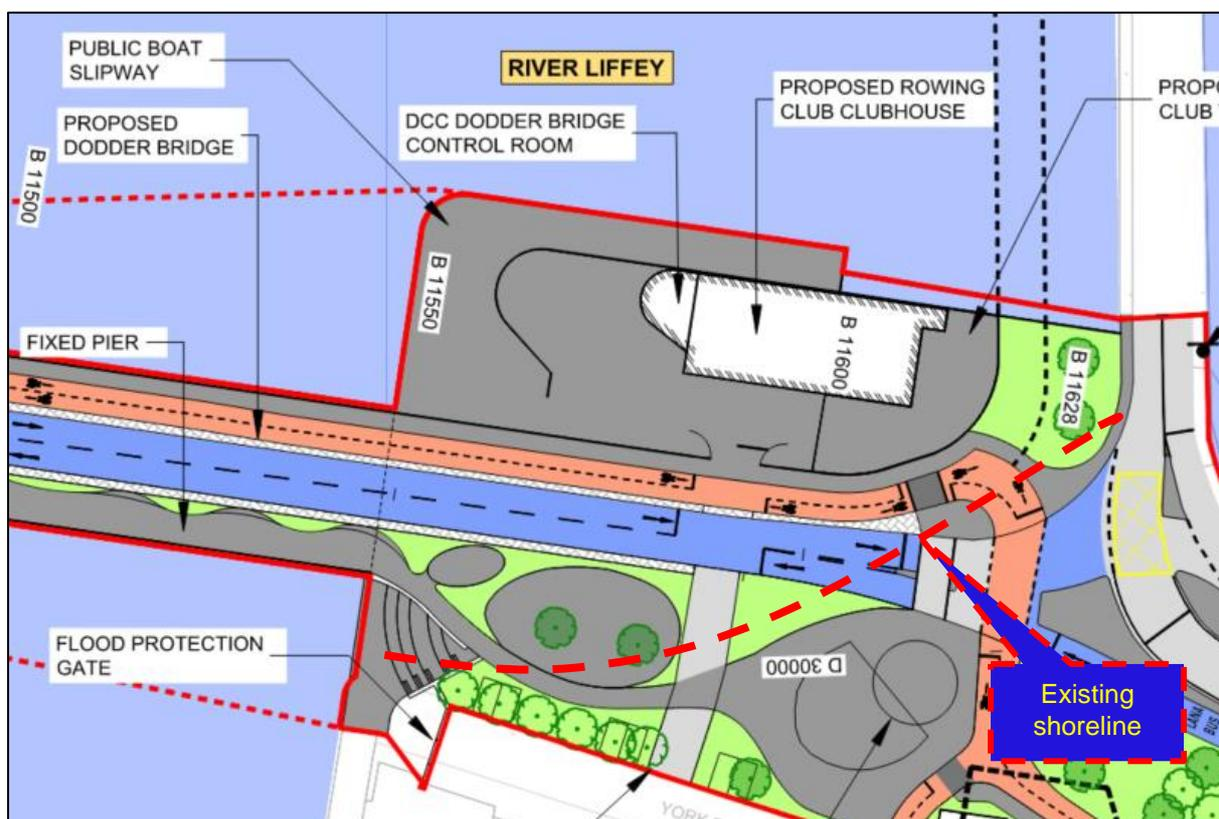
**Figure 3-20b: Proposed Land Reclamation east of the River Dodder Public Transport Opening Bridge at Ringsend**
