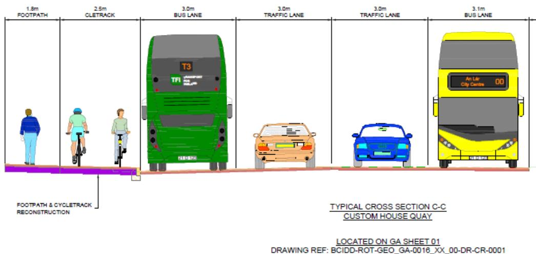
**Figure 3-6b: Proposed Road Cross Section at Custom House Quay West**
