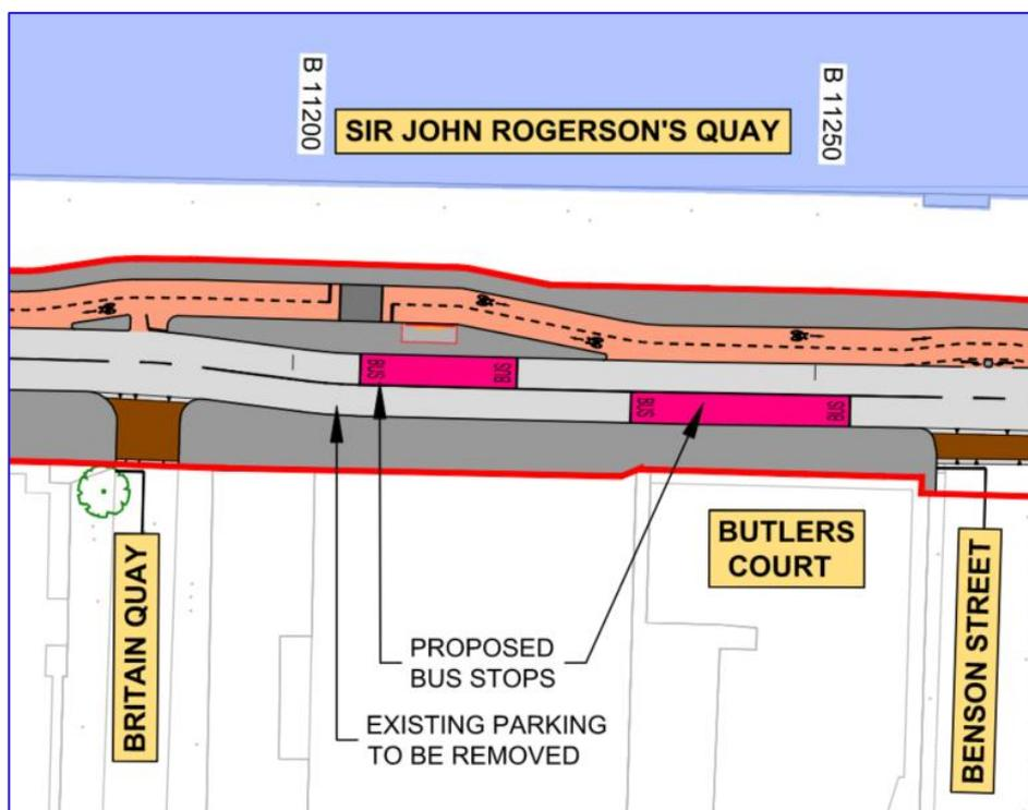
Figure 3-17: Typical proposed layout in Section 1.2B
