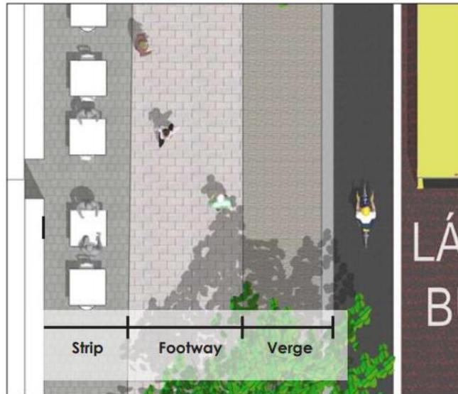
**Figure 4-4: Key components of the footpath**
