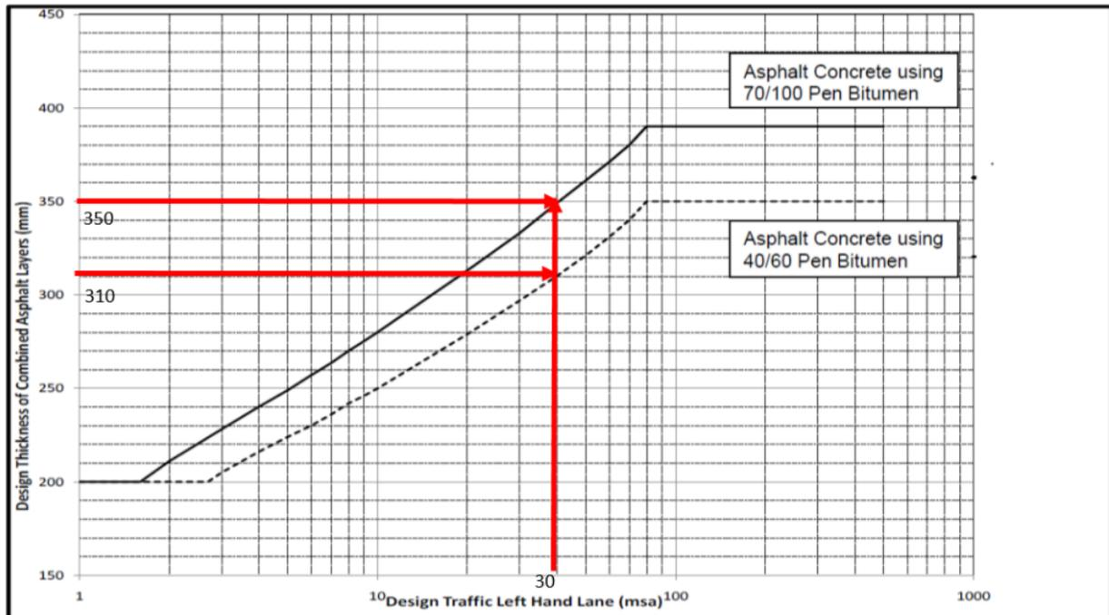
**Figure 7-7: Ringsend to City Centre. Pavement Design Thickness**
