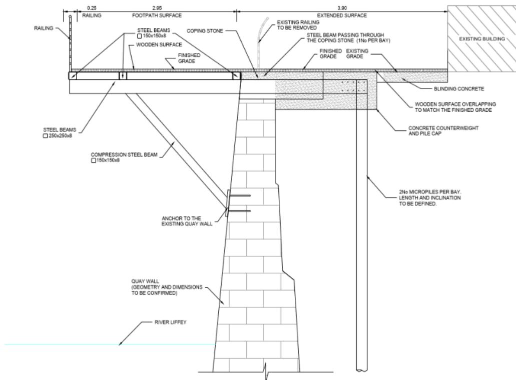
**Figure 8-9: Cross Section Ringsend 02**
