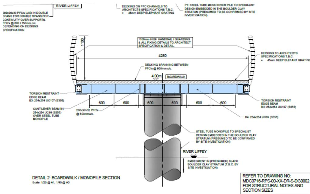
**Figure 8-118: Elevation view Ringsend 04 (Free-standing element)**
