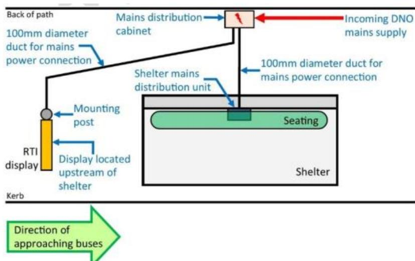
**Figure 12-7: Typical Layout for Bus stop with RTPI Display**
