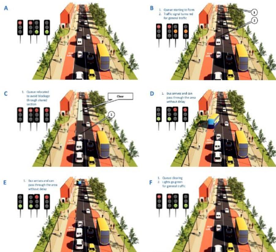
**Figure 12-8: Signal Controlled Bus Priority Schematic Operation**
