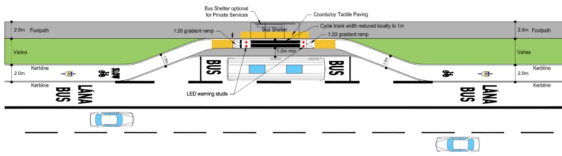
**Figure 4-10: Example of a Layby Bus Stop**
