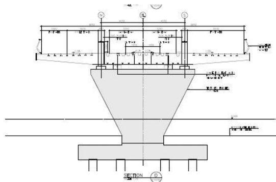
Figure 8-21 Cross Section and Pier Detail
