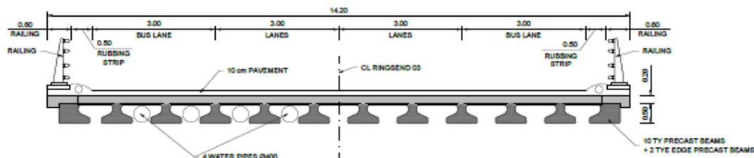
**Figure 8-11: Deck Section Ringsend 03**
