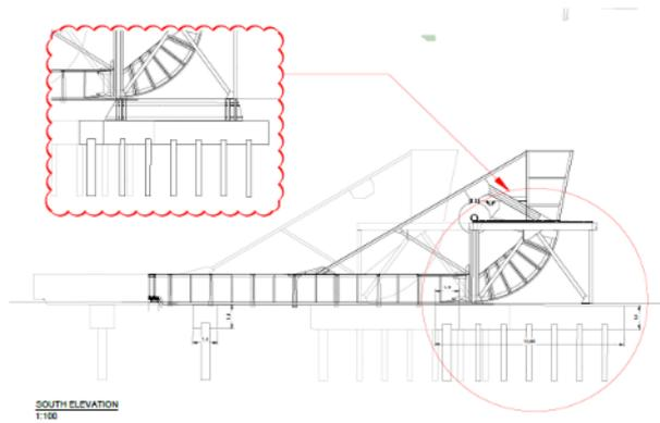
**Figure 8-6: Elevation of Relocated Scherzer Bridges**
