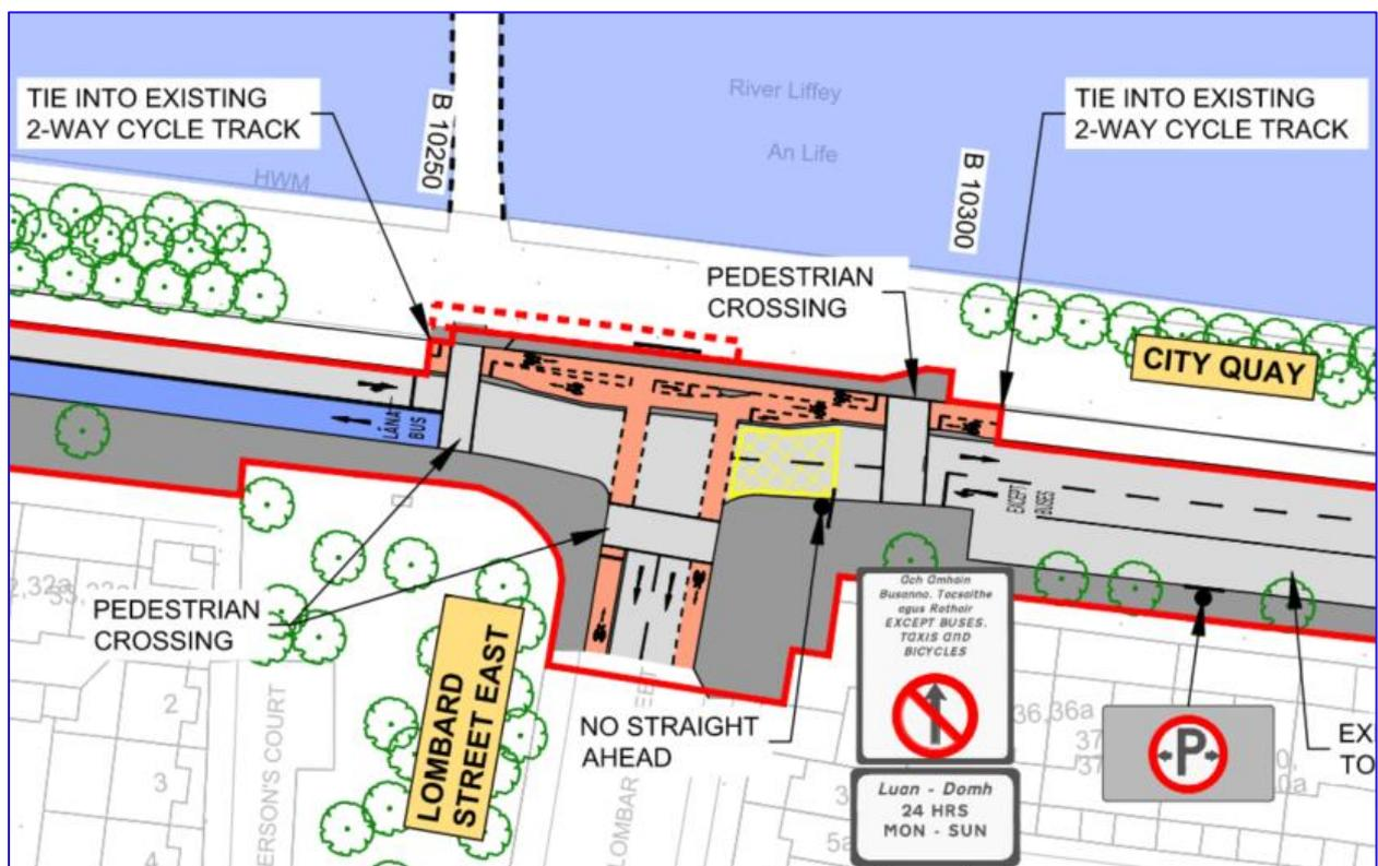
Figure 3-16b: Proposed layout at the junction of City Quay and Lombard Street East
