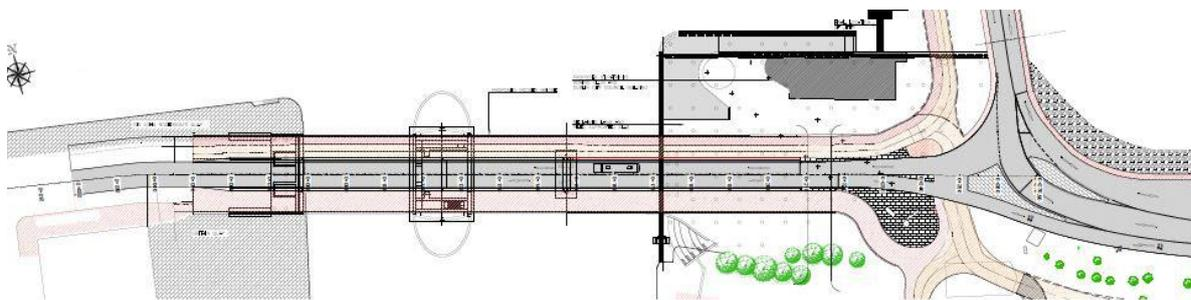
Figure 8-20 Plan of Proposed Dodder Public Transport Opening Bridge
