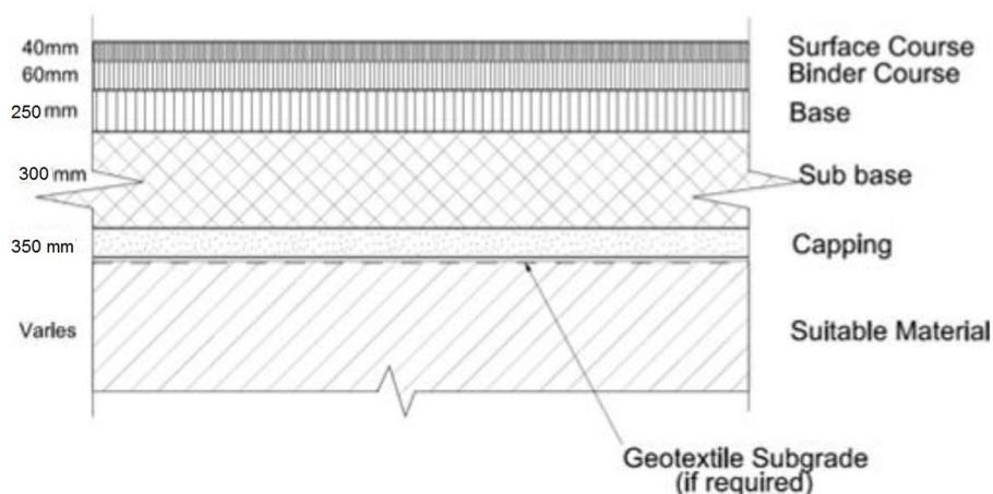
**Figure 7-8: Pavement Structure of Bus Lane. Typical detail**
