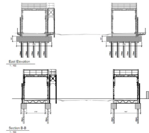
**Figure 8-14: Cross Sections of Relocated Scherzer Bridges**
