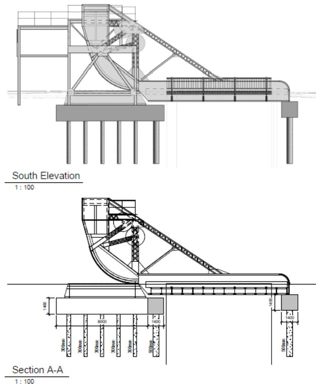
**Figure 8-15: Elevations of Relocated Scherzer Bridges**
