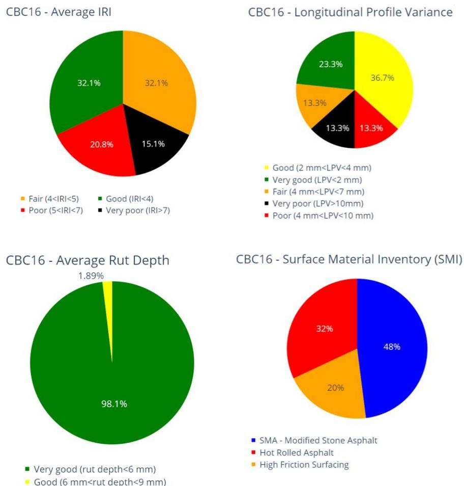
**Figure 7-3: Ringsend to City Centre. IRI, LPV, Rut depth and SMI. Source: RMO dataset**
