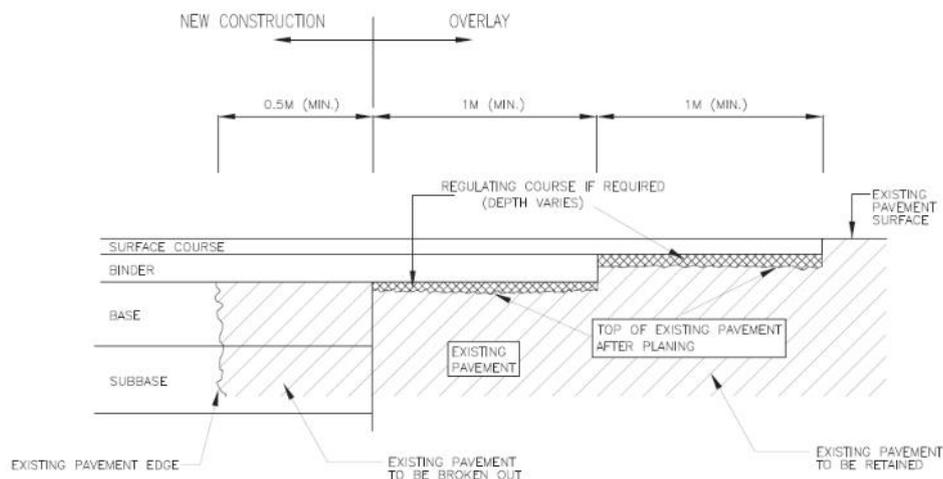
**Figure 7-2: Transversal Joint between new construction and existing road as per CC-SCD-00704-03**
